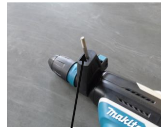
Foam allows for bolt to stay in place.
